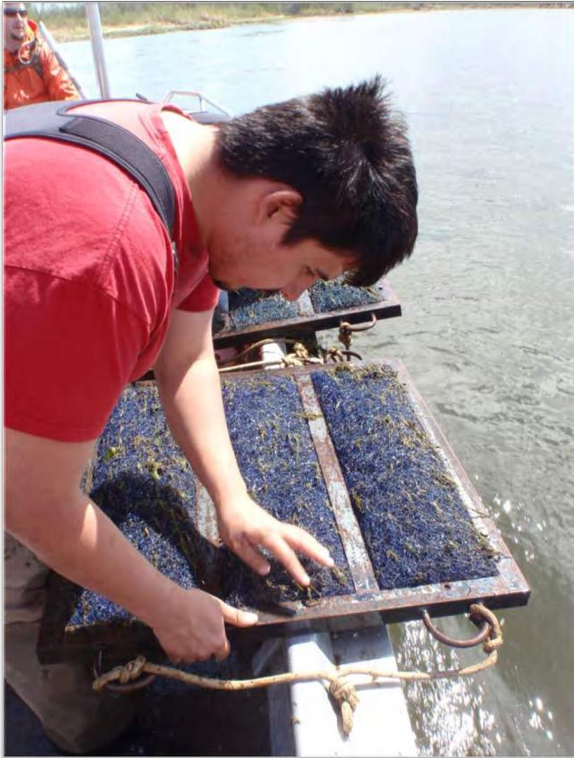
Here a researcher checks large heavy mats that are placed on the river bottom. Sturgeon eggs stick to the mats (as does silt). Eggs on the mats are collected and taken to the hatchery to be raised. The orange buoys you see in the river near the bridge each spring has one of these mats connected to it.
