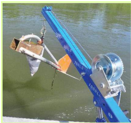
Bedload is assessed using a Helley-Smith sampler, attached to a crane and launched from an anchored boat. Photo by NHC and can be found in their 2014 report.
