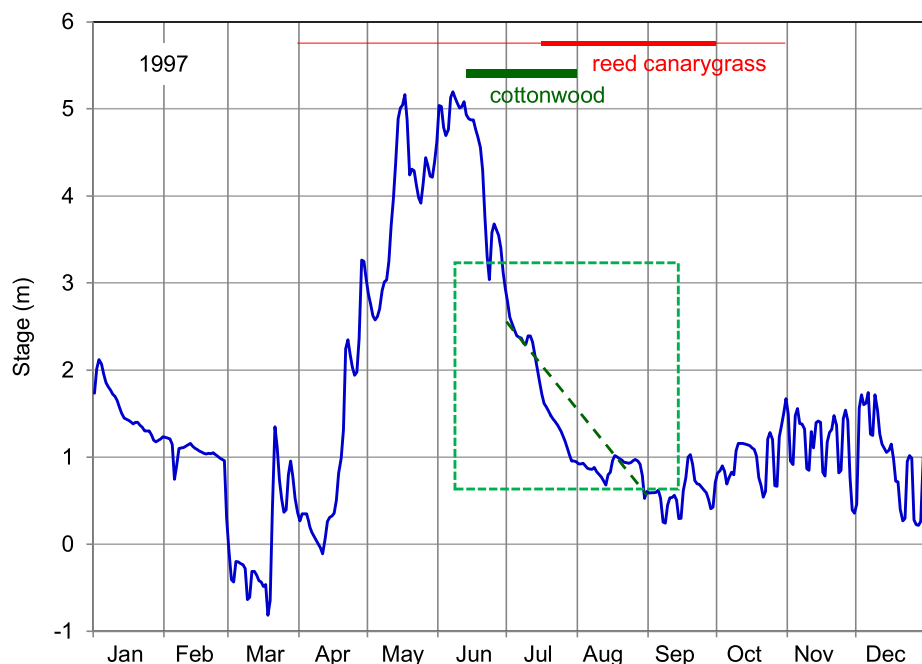
FIGURE 7 Daily hydrographs for 1997 for the Kootenai River at Bonners Ferry, ID, upstream of the meander reach. The green Recruitment Box characterizes favorable conditions for cottonwood colonization and the favorable recession limit is provided by the dashed line ( \sim 3 cm/day or 1 m/month). Typical intervals of seed dispersal for cottonwoods and reed canarygrass (rcg) are displayed—cottonwood seeds have short viability while rcg seeds remain viable for one or more years. [Color figure can be viewed at wileyonlinelibrary.com ]
